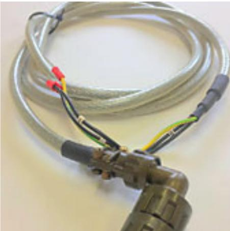
Magnetic pickups (MPUs) are sensors that detect the speed of a turbine. They are the communication link between the engine and governor control.
